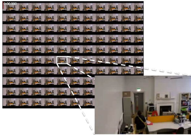
Fig. 4. Panopticon is a video surrogate system that represents an overview of the frames of a video in a grid configuration. Each tile in the grid represents a moving section of video.
